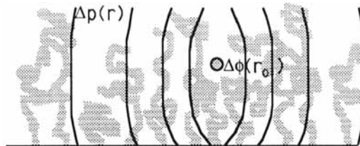
Figure 3 Sketch of a grafted layer with a small region of perturbed density \Delta\phi . Curved black lines suggest pressure response \Delta p .
